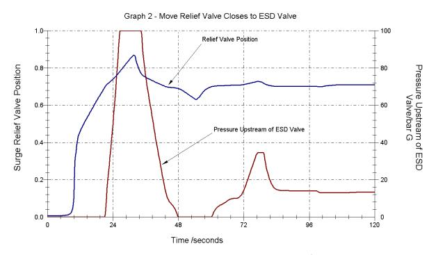
This indicates that the maximum pressure might come down if the valve is made bigger. This is because the calculation shows that the surge relief valve fully opens but is not able to control the pressure.
