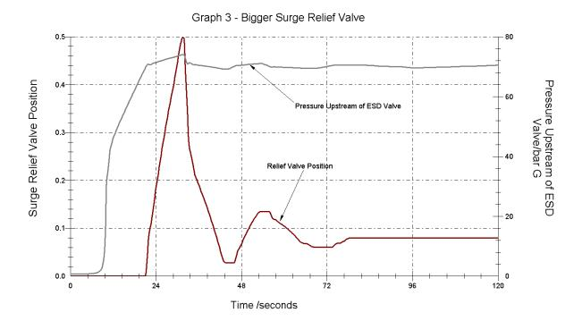
This indicates that the relief valve will remain open as long as the pumps are running. So it is necessary to increase the set point of the surge relief valve.
