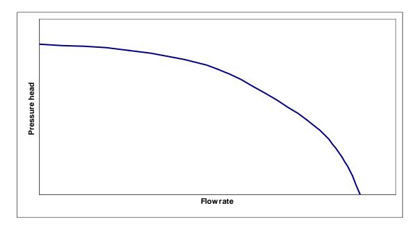
This model is in adequate for modelling pump trip events, especially for large pumps. When a pump trips the pressure downstream of the pump can become a vacuum pressure. Furthermore, the flow can reverse and the pump can rotate backwards. In order to model this phenomenon PIPENET offers a model called the "Turbo Pump" model. This can model the behaviour of the pump in all the 4 quadrants of operation. The pump curve for a Turbo Pump is shown below and it covers all 4 quadrants.
