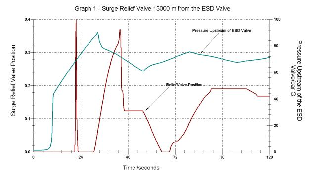
This indicates that the closer the Relief Valve is to the ESD Valve the better
