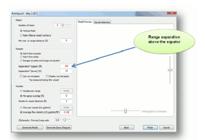
The library had 3 nozzles in this case. Our choice of nozzle N-2 below is arbitrary just to illustrate the dialog box. Note that the total flow for the chosen nozzle divided by the surface area of the vessel is  $439.5/(\pi \ [48] ^2) = 0.0607$  gpm ft-2 which is significantly higher than 0.05. We will see why this is later on.
