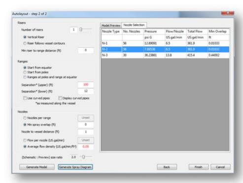
By generating a new spray diagram the following can be obtained:
