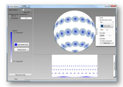
The nozzle cones are shown and they are extended to full size so that they touch the sphere. We see that, although the nozzles are now utilizing 100% of their flow, there are now large areas of unprotected surface. So, increased efficiency and reduced flowrate have been obtained at the cost of increased number of nozzles and poor vertical coverage. Furthermore, the nozzles may be working below the vendor recommended minimum pressure.
