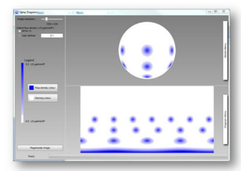
The same spray diagram with the sphere rotated to show the plan view results in the following. This diagram also shows the spray cone.
