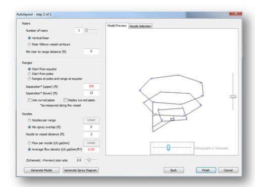
Generating the spray diagram for the model results in the following.
